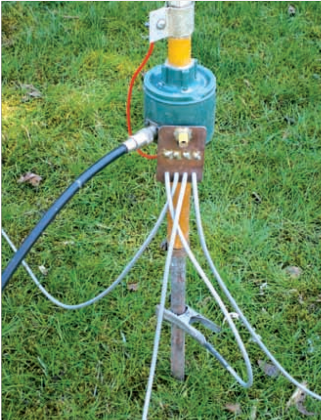
Fig. 2: The base, showing the ground connecting leads. They connect to the screen of the coaxial cable feeder.
