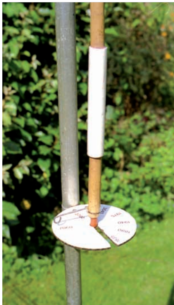
Fig. 4: The calibrated band-indicator plate with the bamboo stick used to operate the band-switch.
