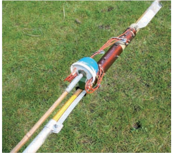
Fig. 3: The mid-antenna mounted band-change switch.
